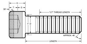
Head markings may vary slightly depending on manufacturing practice. Diamond knurls, UNBRAKO, and UNB are recognized identifications for 1/4" diameter and larger.
